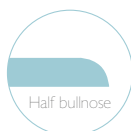
Step tread 20mm Typically 600 x 100mm
